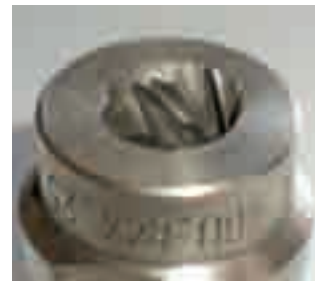
Figure 19: Wear of a full cone nozzle
