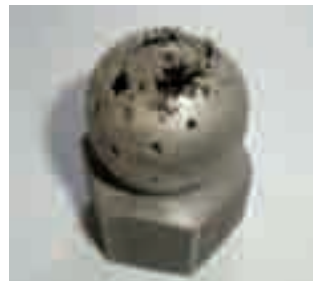
Figure 18: Chemical corrosion of a spray ball
